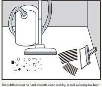
The subfloor must be hard, smooth, clean and dry, as well as being free from defects and fit for purpose. When required, scrape off and remove old adhesives and loose lay-ing leveling compound. Make sure the subfloor is flat and free from chemical substances and other contamination.
